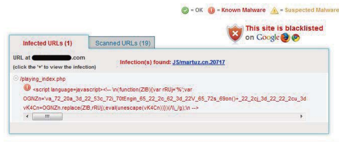
FIGURE 4: EXAMPLE OF MARTUZ ATTACK (VARIANT OF GUMBLAR), WHICH USED STOLEN FTP CREDENTIALS TO ATTACK LEGITIMATE WEBSITES
